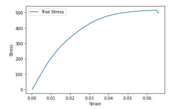
As this graph is a non-linear one, yield stress could be determined by the offset method. So we calculated the initial slope of the graph and plotted a line having the same slope and x-intercept as 0.2% of maximum strain.
