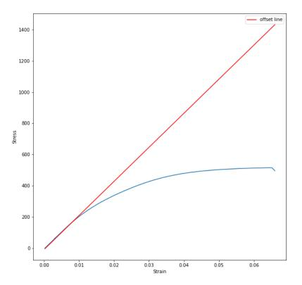
The point where the two graphs intersect correspond to the stress value of 165.8250061 which becomes the yield stress of the graph. After generating the yield stress we try to fit the plastic region of the graph into a polynomial function  $A + B * X^n$ , where X corresponds to the strain part of the graph. So, for this we firstly generate 150 random values of A in between 0 and 515, 150 random values of B between 0 and 3,500 and 50 evenly spaced values of n between 0 and 3.
